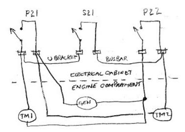
So where does the extra cable go? Why is there a 2:1 difference in the apparent load between engine 1 and engine 2? What is the actual resistance of a traction motor? Can the hypothicated switching circuit be verified/corrected? If verified, there will be two options: 1) a push-on/push-off switch on the console; 2) rewire the V1 relay to be in "parallel" as the default rather than in "series".
